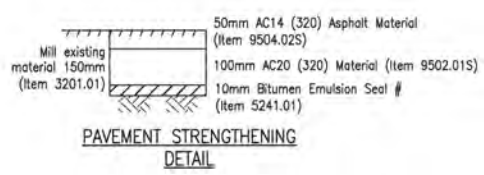
PAVEMENT RESURFACING DETAIL
