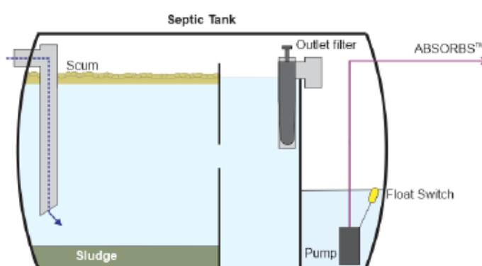
Figure 3 Schematic of your pre-treatment system
