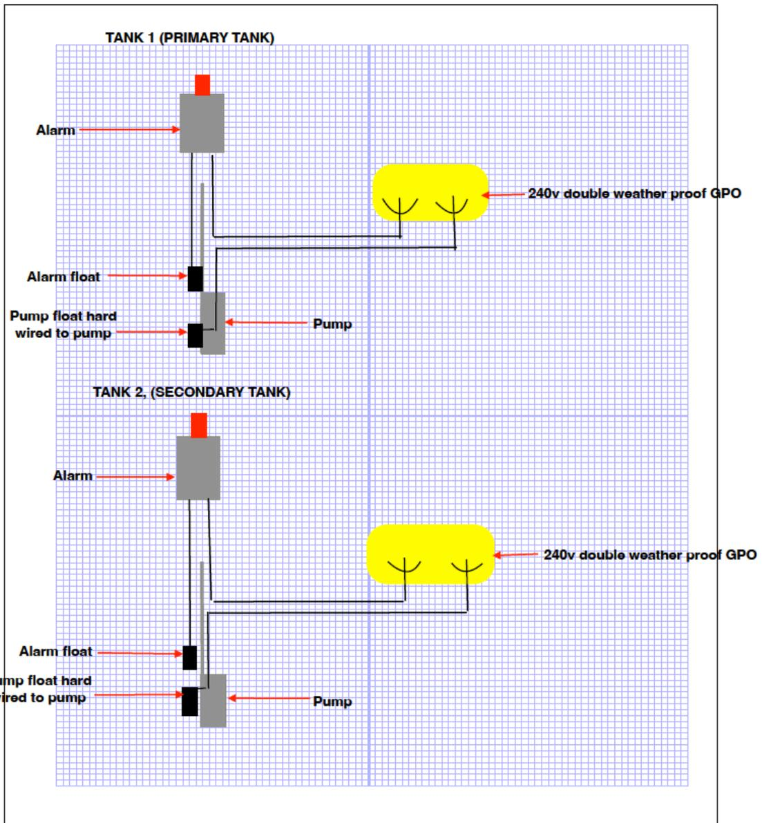
Attachment 4 – Wormsmart WSP1500PF System Schematic
